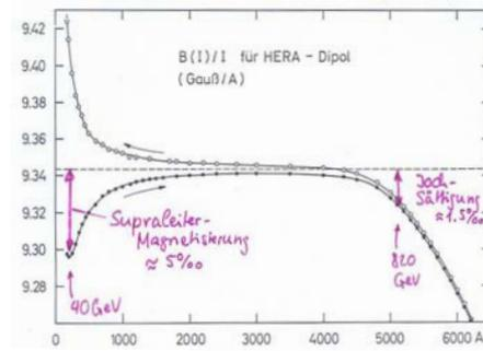
Dipole field  $B_1$  at injection 0.5% lower
