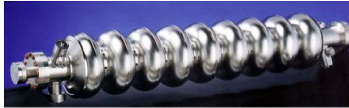
Cavity made from ultrapure niobium
