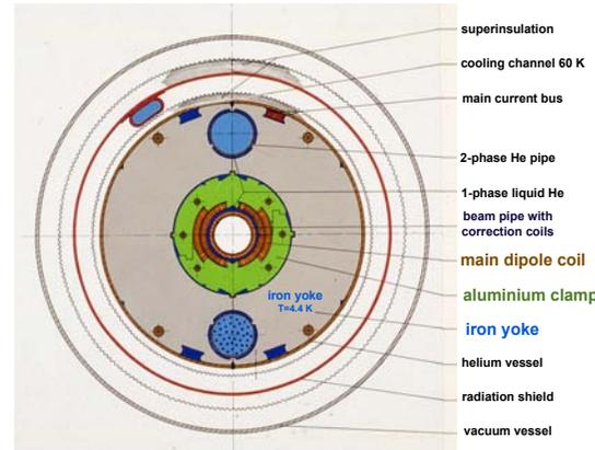
Cross section of HERA dipole:
